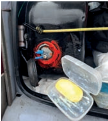
Fuel trouble: a leaking fuel sender was cured with red gunk and Clive's bath soap.
