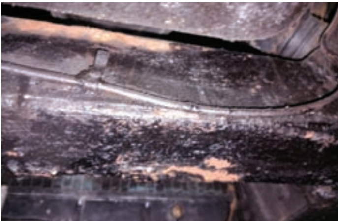
The front crossmember suffers from the lack of an engine oil leak.
