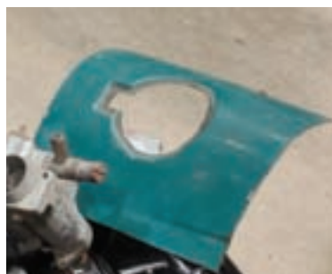
Mk3 Fuel Cap recessed section cut from a rear wing.
