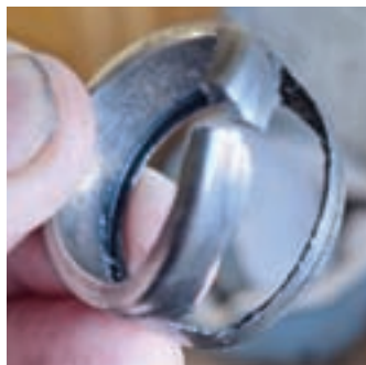
Remains of inner driveshaft bearing.
