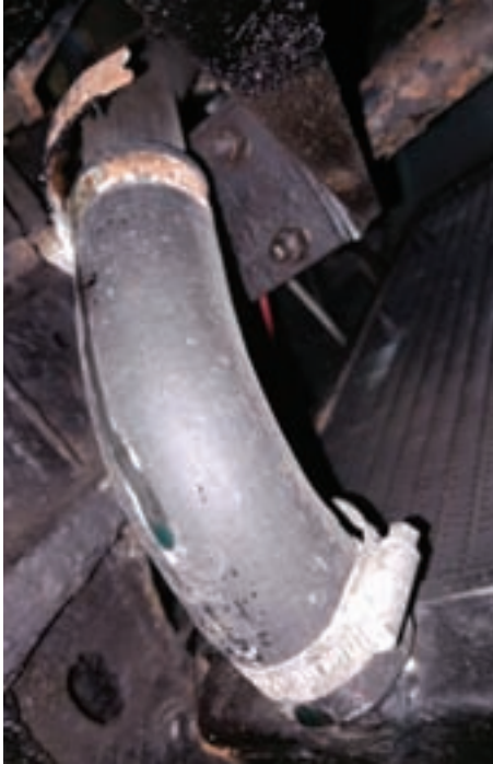
A seeping coolant hose was found and the clip tightened.
