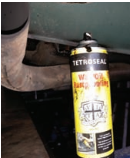
Bernard also used an aerosol of Tetroseal wax oil rust protection to get in the nooks and crannies.
