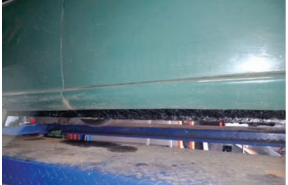
This is the bottom of the sill after being treated.
